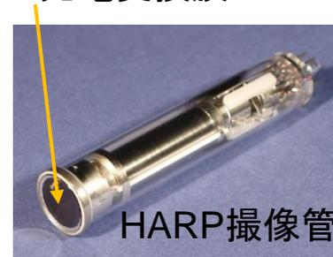
HARP: High-gain Avalanche Rushing amorphous Photoconductor
